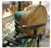
I cleaned up my wood pile the other day and found a dried round that was 18 inches - larger than my lathe capacity. My lathe is a Grizzly model G0462 and the inboard capacity on it is 16 inches. I decided to turn the piece with an outboard setup. I mounted the piece with my chuck ring and attached it to my SuperNova 2 chuck, rearranged my banjo and tool rest and got to work. I established my foot and rounded over the outside of the bowl. I had in
