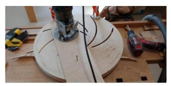
The photo to the left shows the routing process about halfway through, and the one below shows the same level of completion without the trammel base and router in place.
