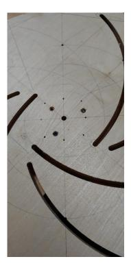
To compete the chuck after routing out the arcs, do the following steps. First, drill a series of finger holes along the outer edge. You can see these in the photo below. Drill them all the way through both disks, sand them, and if you like, round over the edges with a palm router and a 1/8" roundover bit. Here's a close-up:
