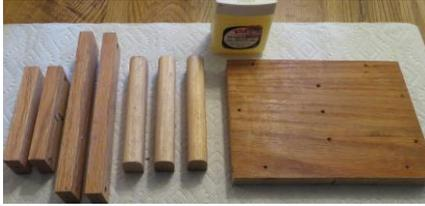
2 Cover your pieces in petroleum jelly on all sides. This helps to keep the silicon from sticking to the mold.
