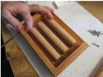
4 Squeeze in the silicon sealant making sure to get it into all the nooks and crannies so you won't have any voids when you remove the silicon mold.
