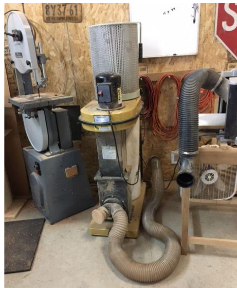
(Below) This shows Bruce's dust collector on his lathe. The wire screen keeps tools and other objects from getting sucked in to his powerful system which is on the other side of a wall which keeps the noise to a minimum.
