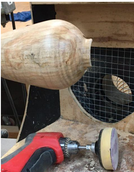
(Below) This shows Bruce's dust collector on his lathe. The wire screen keeps tools and other objects from getting sucked in to his powerful system which is on the other side of a wall which keeps the noise to a minimum.
