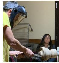
Dan cautioned us the beginning of the drilling must be smooth as any oscillations will get worse with depth
