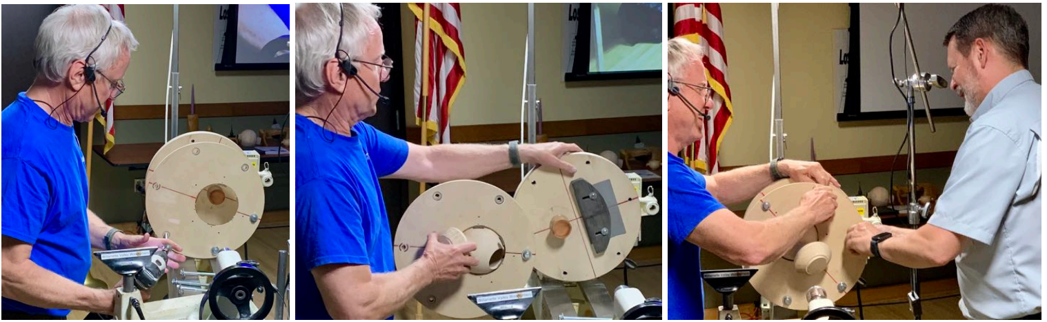
Above: opening jig, open jig with counterweight visible, Darcy stepping up for the tedious threading of bolts... Below: seeing the “ghost” and where the drill will go for the spout, drilling spout (clear threads often!)
