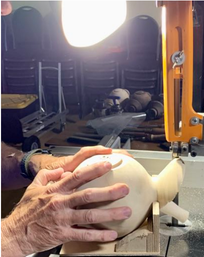
Above: various sized sleds, placing pot in sled Below: cut off sides of spout, then base leaving material for shaping (not too much...)
