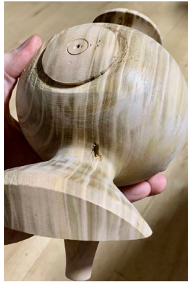
Above: the “mistakes”-too short, unaligned, drill through side, unsupported spout
