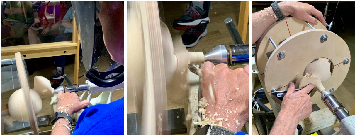
Above: cone center in drilled spout, turning spout Below: spout turning, refine the tip at this point
