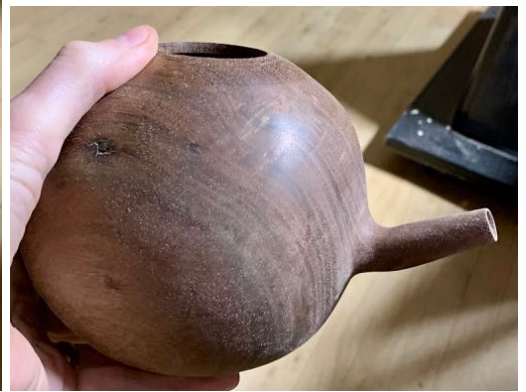
Above: the “mistakes”-too short, unaligned, drill through side, unsupported spout
