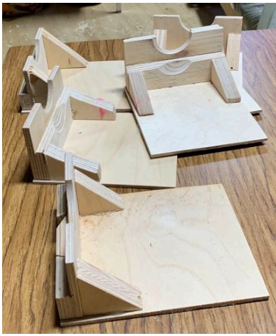
Above: various sized sleds, placing pot in sled Below: cut off sides of spout, then base leaving material for shaping (not too much...)
