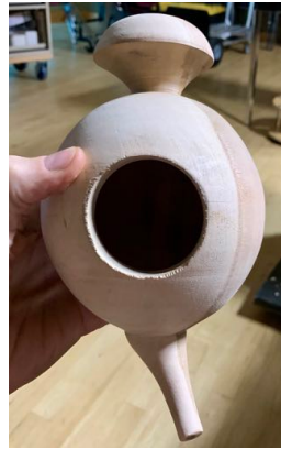
Above: the “mistakes”-too short, unaligned, drill through side, unsupported spout
