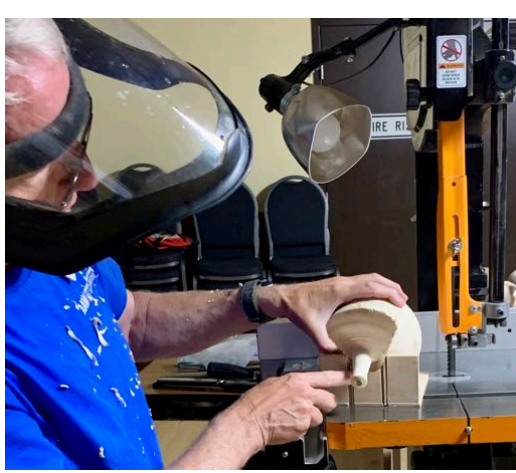
Above: various sized sleds, placing pot in sled Below: cut off sides of spout, then base leaving material for shaping (not too much...)
