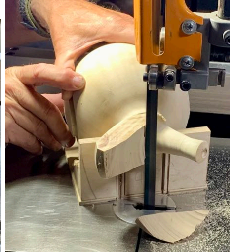
Above: various sized sleds, placing pot in sled Below: cut off sides of spout, then base leaving material for shaping (not too much...)
