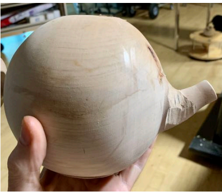
Above: the “mistakes”-too short, unaligned, drill through side, unsupported spout
