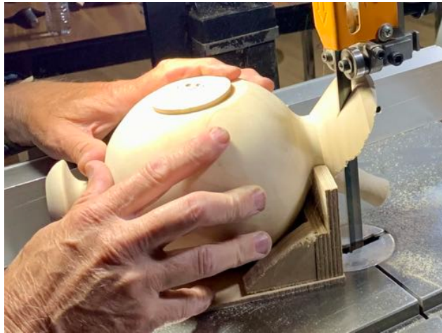
Above: various sized sleds, placing pot in sled Below: cut off sides of spout, then base leaving material for shaping (not too much...)
