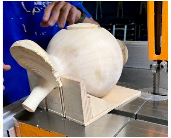
Above: various sized sleds, placing pot in sled Below: cut off sides of spout, then base leaving material for shaping (not too much...)
