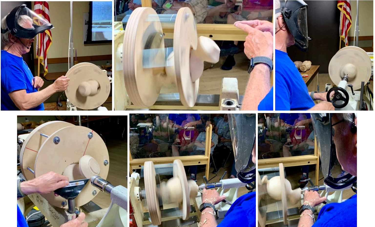
Above: cone center in drilled spout, turning spout Below: spout turning, refine the tip at this point
