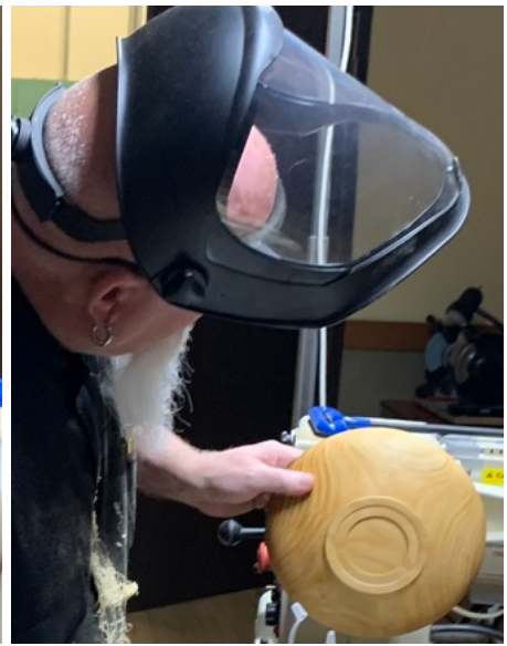
Above: Brett used a 3 sided pointed tool to refine the foot and mortis to match the jaws he would use to hold the piece when he reversed it.
