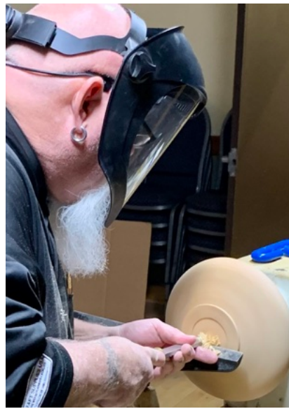
Above: Brett used a 3 sided pointed tool to refine the foot and mortis to match the jaws he would use to hold the piece when he reversed it.
