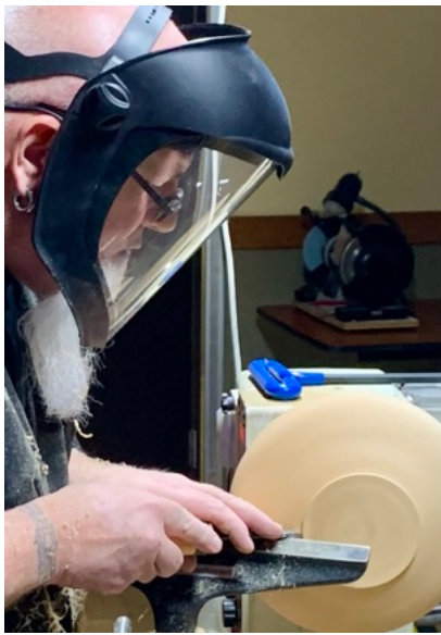
Above: Brett used a 3 sided pointed tool to refine the foot and mortis to match the jaws he would use to hold the piece when he reversed it.
