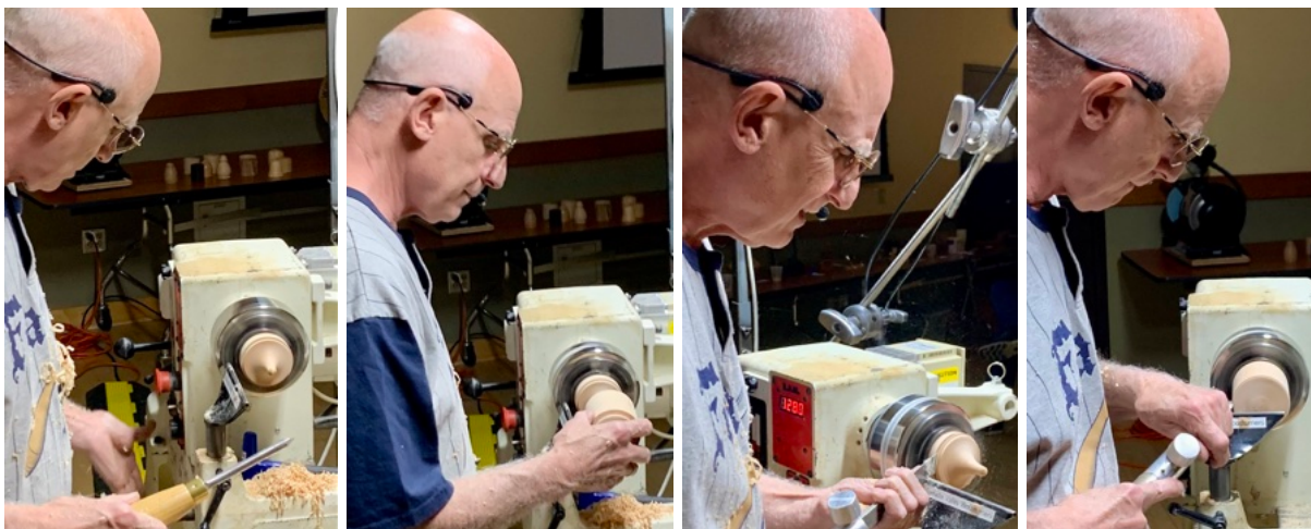
Above: Sneaking up on making a tight fit (did have to use a paper towel; said it's common) and part off. Right and below: Press fit funnel into body and cut base of funnel. Terry showed a dedicated epoxied drill in a handle and a hand held drill with a chuck.
