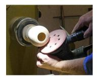
Sand the inside using a hemostat clamping sandpaper around a wad of cloth. Move the angle of the sandpaper to match the angle of the inside contour. Sand the outside with a random orbit sander hooked up to a vacuum.
